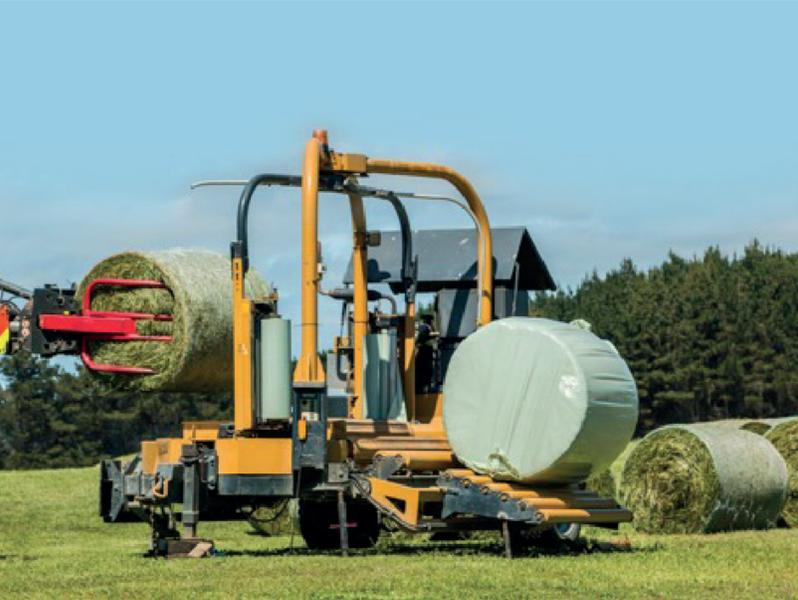
*Silage is a feed obtained as a result of fermentation (souring) of water-rich feeds under the influence of lactic acid bacteria in an airless environment. It is the process of wrapping the feed product with cling film via a machine after it has been reduced to a certain size and baled.*
